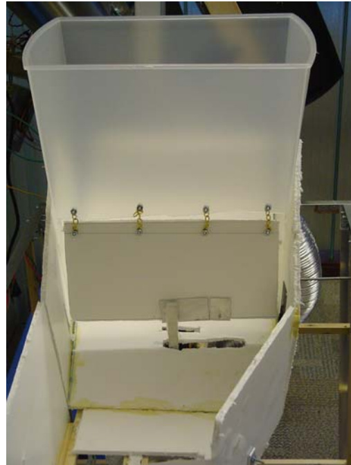
Fig. 2. (right) The loading bin with servo motor-controlled gate.
